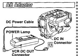
Connect AC Adaptor VCR DC OUT to Camcorder DC IN with supplied DC Power Cable.
