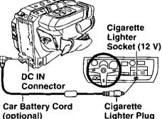
Connect PV-C16 <u>Car Battery Cord</u> (optional) to <u>Camcorder DC IN</u>.
